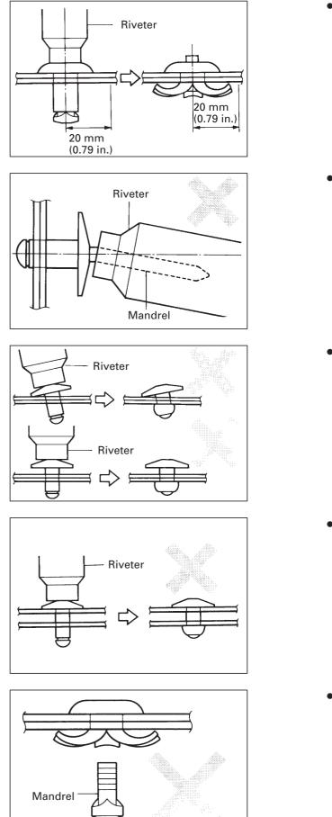
• T-Rivet with ø6.4 mm: Do not place your hands or the wire harness within a radius of 20 mm (0.70 in.) from the rivet, as the rivet is cut and opened in this area.
