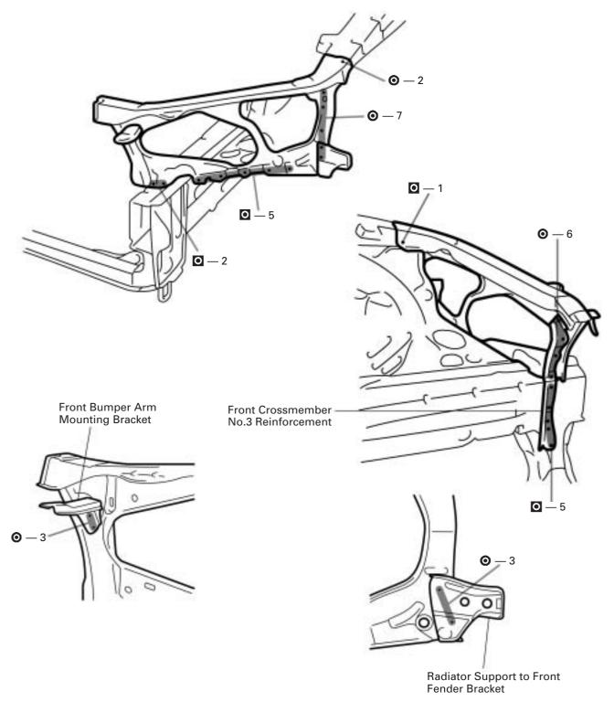
1. Temporarily install the new parts and measure each part in accordance with the body dimension diagram.
