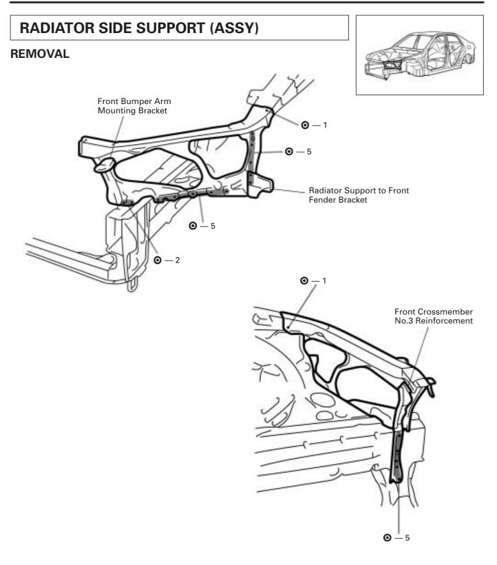
1. Replace the radiator support to front fender bracket, front bumper arm mounting bracket and front crossmember No.3 reinforcement at the same time.
