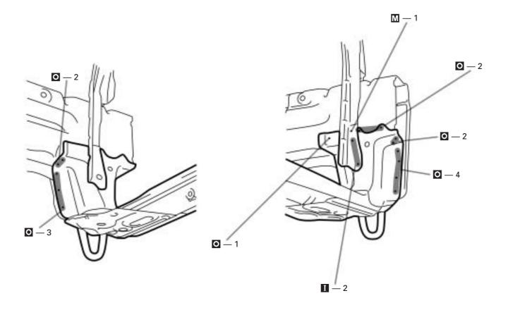
Temporarily install the new parts and measure each part in accordance with the body dimension diagram.
