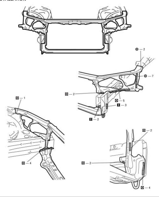
Temporarily install the new parts and measure each part in accordance with the body dimension diagram.
