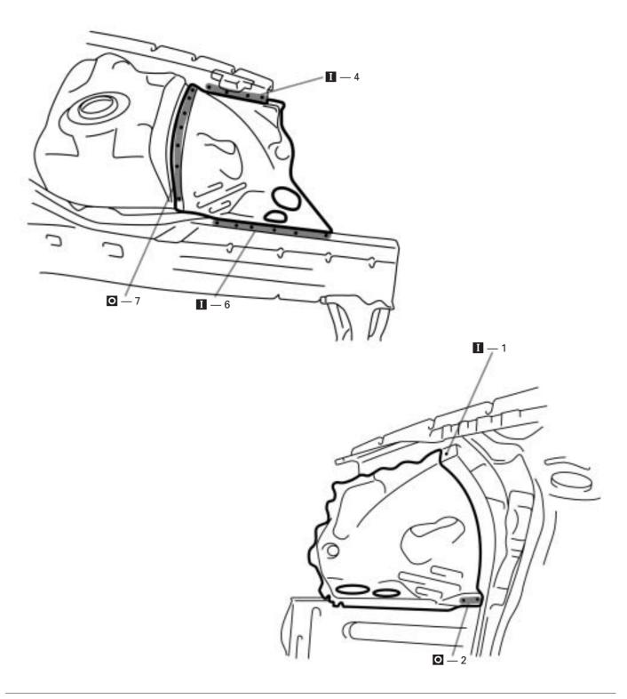
Temporarily install the new parts and measure each part in accordance with the body dimension diagram.
