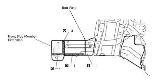
Temporarily install the new parts and measure each part in accordance with the body dimension diagram. **- MEMO -**
