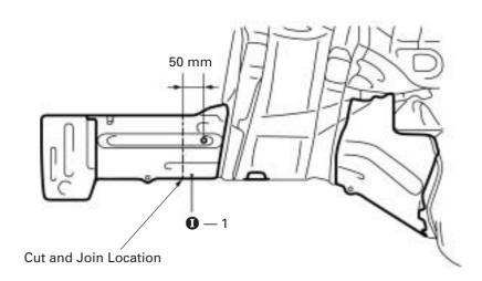
1. Cut and join the parts at the locations as shown above.
