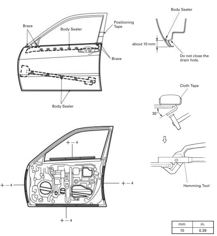
1. Before temporarily installing the new parts, apply body sealer to the reinforcement, side impact protection beam and back side of the new parts.
