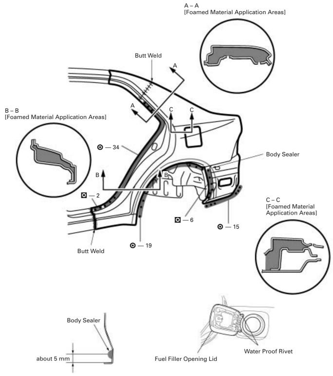
1. Before temporarily installing the new parts, apply body sealer to the wheel arch.
