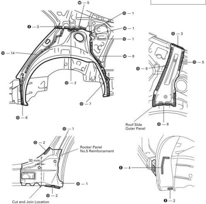
1. Remove the roof side outer panel and rocker panel No.5 reinforcement at the locations shown above, and remove the quarter wheel housing outer panel.
