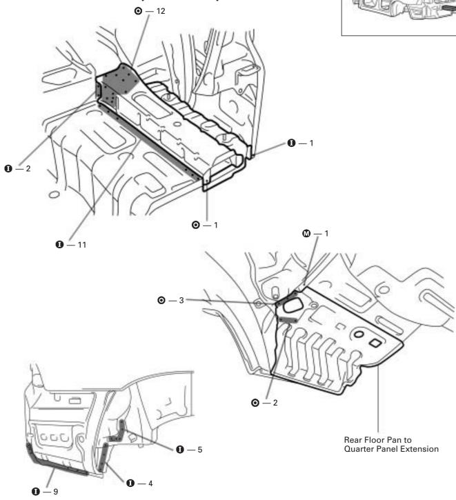
Replace the rear floor pan to quarter panel extension at the same time as the rear floor side rear member.
