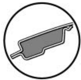
A - A [Foamed Materials Application Area]
