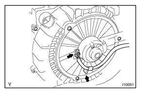
(b) Remove the wire harness clamp and disconnect the connector.
