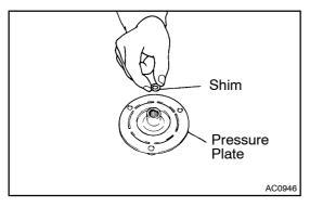
(d) Remove the shims from the pressure palate.
