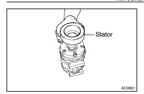
(c) Remove the stator.
