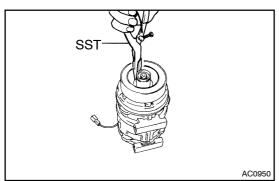
(b) Using SST, remove the snap ring. SST 07114-84020
