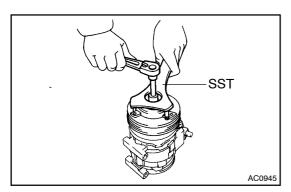
(c) Using SST and socket wrench, remove the pressure plate.
