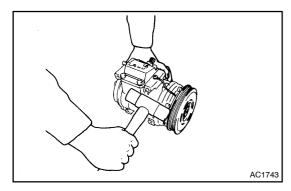
(b) Using a plastic hammer, tap the rotor off the shaft.
