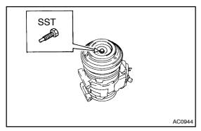
(b) Install SST on the pressure palate. SST 07112–66040
