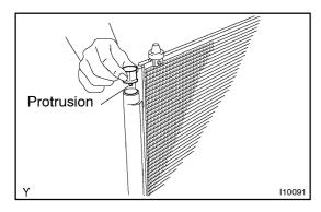
(e) Insert the filter into the modulator.
