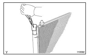
(c) Using pliers, remove the dryer.
