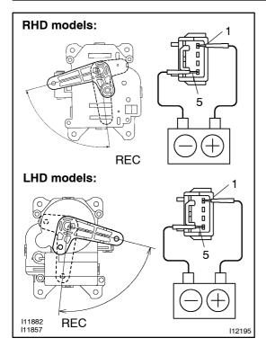
(b) Connect the positive (+) lead from the battery to terminal 1 and negative (-) lead to terminal 5, then check that the arm turns to "RECIRC" side smoothly.
