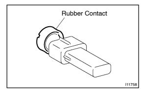
NOTICE: Do not let any oil, dirt or foreign object attach on the rubber contact part.
