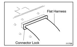
(c) Release the connector lock and pull out the flat harness. **NOTICE:**
