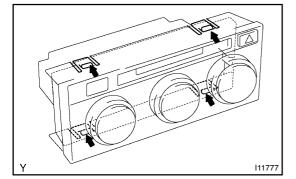
(b) Using a screwdriver, release the 4 claws and pull out the A/C amplifier.
