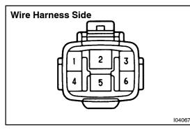
4. **INSPECT HEADLIGHT CLEANER RELAY CIRCUIT** Disconnect the connector from the relay and inspect the connector on wire harness side, as shown.
