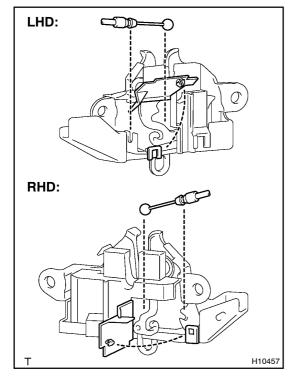
(c) Using a screwdriver, open the cover, then disconnect the hood lock control cable.
