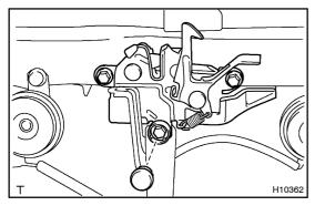
(b) Install the hood lock with the 3 bolts.
