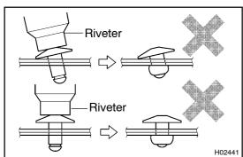
Do not tilt the riveter and disconnect the rivet from the material while handling a riveter, as the materials are not tightened firmly.
