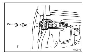
(c) Install the outside handle with the key cylinder to the door panel with the 2 bolts.
