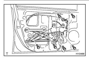
(a) Install the window regulator with the 6 bolts.
