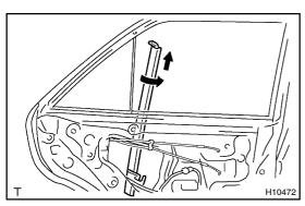
(c) Rotate the division bar 90° and pull it upward as shown in the illustration.
