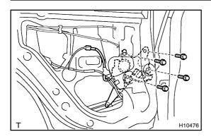
(a) Install the window regulator with the 4 bolts.
