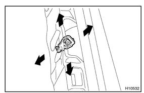
(c) Using a hammer and brass bar, tap the striker to adjust it.
