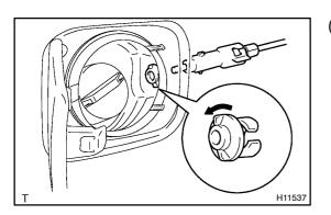
(b) Rotate the retainer left to disengage the lock, then pull it out.
