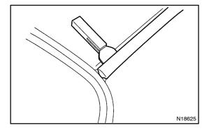
(c) Using a scraper, pull off the roof drip side finish moulding from the front end and rear end.
