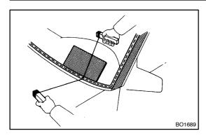
(d) Cut the adhesive by pulling the piano wire around it.
