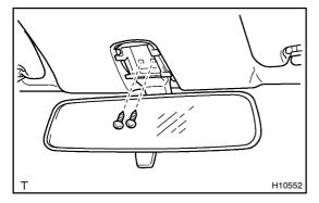
(b) Remove the 2 screws and inner rear view mirror.
