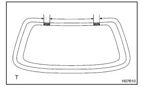
(e) Let the piano wire pass as shown in the illustration, cut off the adhesive sticking to the stoppers.
