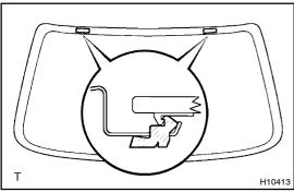
(f) Disengage the stoppers, then remove the glass.
