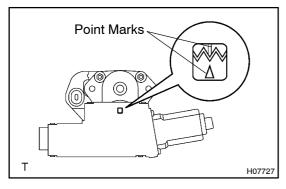
(c) Turn the drive gear to align the point marks as shown in the illustration.
