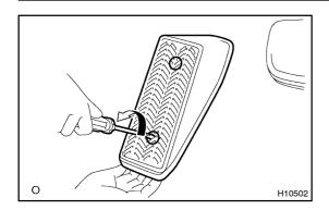
(b) Using a screwdriver, remove the foot rest as shown in the illustration.
