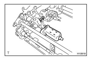
**3. INSTALL FRONT VERTICAL MOTOR** Connect the front vertical motor, then install the 2 screws.
