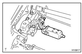
**4. INSTALL LIFTER MOTOR** Connect the lifter motor, then install the 2 screws.
