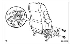
(c) Remove the 4 seatback assembly set bolts.
