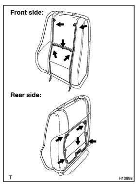
(e) Remove the 10 hog rings, headrest supports and seatback cover as shown in the illustration.
