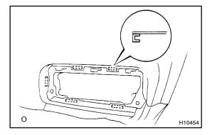
(d) Unlatch the seatback cover hooks circumference of the side airbag assembly.
