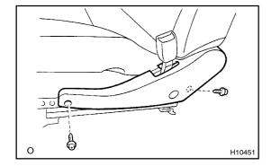
**10. INSTALL FRONT SEAT CUSHION INNER SHIELD** Install the front seat cushion inner shield with the 2 screws.
