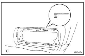
(c) Hook the seatback cover hooks through the holes in the circumference of the side airbag assembly.
