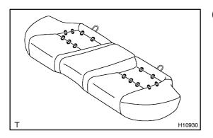
(b) Remove the hog rings and seat cushion cover on the front of the seat cushion assembly.
