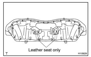
(b) Install new hog rings to the back of seat cushion assembly.
