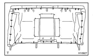
(c) Install new hog rings on the back of seatback assembly. HINT:
