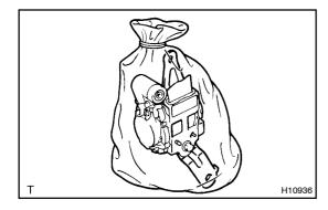
(e) Dispose of front seat outer belt (with seat belt pretensioner).
