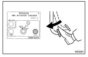
(e) Push the POWER switch and check that the brake pedal does not go down.
