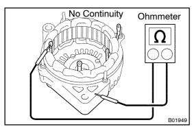
(b) Check the stator for ground.Using an ohmmeter, check that there is no continuity between the coil lead and drive end frame.
