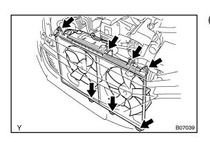
(f) Remove the 6 bolts and electric cooling fan.
