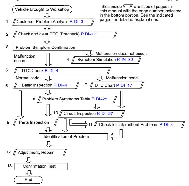
When not using hand-held tester, troubleshoot in accordance with the procedure on the following page.
