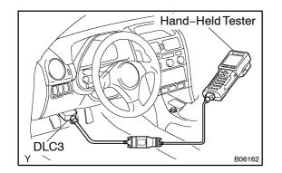
To check the DTCs, connect the OBD scan tool or hand-held tester to the Data Link Connector 3 (DLC3) on the vehicle. The OBD scan tool or handheld tester also enables you to erase the DTCs and check freezed frame data and various forms of engine data. (For operating instructions, see the OBD scan tool's instruction book.)
