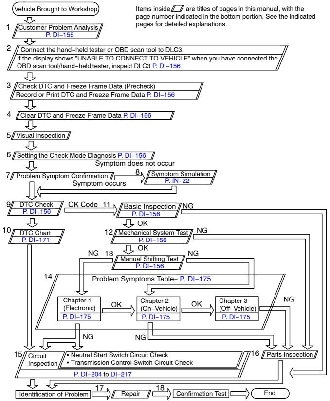
When not using hand-held tester, troubleshoot in accordance with the procedure on the following pages.
