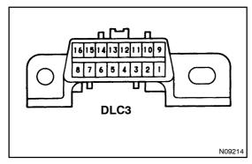
(4) Read the DTC indicated by the number of times the PWR indicator light blinks.
