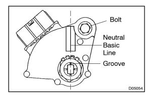
(f) Inspect and adjust the neutral start switch. Check that the engine can be started with the shift lever only in the N or P range, but not in other ranges.
