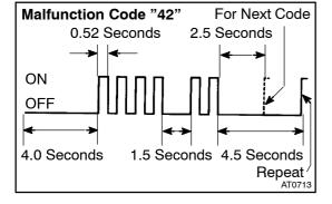
(2) The malfunction code is indicated, as shown in the chart on the left (DTC "42" is shown as an example).
