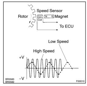
The speed sensor detects wheel speed and sends the appropriate signals to the ECU. These signals are used for control of both the ABS & TRC control system. The front and rear rotors each have 48 serrations.
