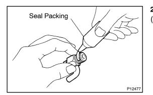
**INSTALL ENGINE COOLANT DRAIN UNION** 22. Apply seal packing to 2 or 3 threads. Seal packing: Part No. 08826-00100 or equivalent
