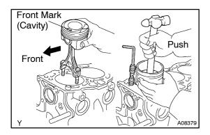
(b) Using a piston ring compressor, push the correct numbered piston and connecting rod assemblies into each cylinder with the front mark of the piston facing forward.
