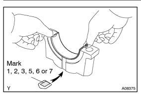
(b) Align the bearing claw with the claw groove of the main bearing cap, and push in the 7 lower bearings.
