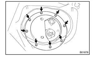
(d) Install the fuel tank vent tube set plate with the 8 bolts.
