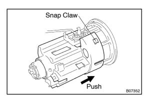
(b) Push the fuel suction support, and attach the 4 snap claws to the claw holes.
