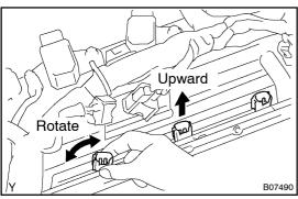
(g) Check that the injectors rotate smoothly.
