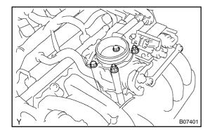
(f) Remove the 2 bolts, 2 nuts, throttle body and gasket from the intake manifold.
