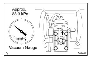
(b) Rapidly depress the accelerator pedal to fully open position and check that the vacuum gauge needle momentarily fluctuates approx. 33.3 kPa (250 mmHg, 9.84 in.Hg) or more. (The actuator rod is pulled down.)
