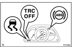
(4) Press the TRC cut switch to turn the TRC to the operative mode and check that the TRC OFF indicator light goes off.
