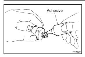
(i) Apply adhesive to 2 or 3 threads of the oil pressure switch. **Adhesive:**
