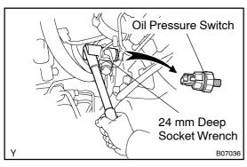
(d) Using a 24 mm deep socket wrench, remove the oil pressure switch.
